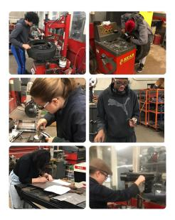
Drilling and tapping photos: at this station students went through the process of correctly identifying the size 3 shop fasteners, selecting a drill bit and tap size using the drill/tap chart, and creating the threads within an aluminum blank. This skill is necessary when repairing or making threads in such items as cylinder heads.
