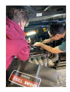
In our automotive classes students performed an electrical software diagnostic to figure out why the check engine light was intermittently triggering on. Upon inspection, students isolated the issue to the engine's valve cover gasket leaking. Students are installing the new engine valve cover gasket in the picture.
