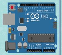
itself can power external devices with a 5-volt power supply, and ground terminals through its 5-volt and ground pins. Through these pins the power and ground rails of the breadboard are powered.
