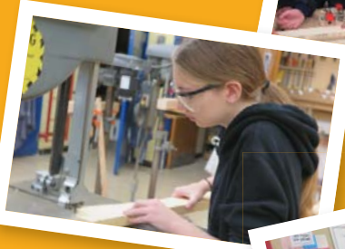
Rough cutting curved rails on the band saw
