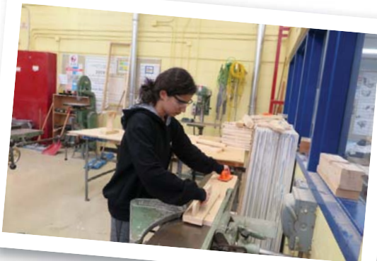
Joining one face of rough sawn pine for the chair leg
